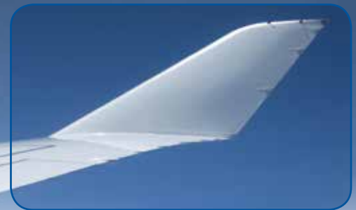
Winglets increase the lift generated at the wingtip by smoothing the airflow across the upper wing side near the tip. Winglets also reduce the lift-induced drag caused by wingtip vortices, improving the lift-to-drag ratio of the aircraft.
